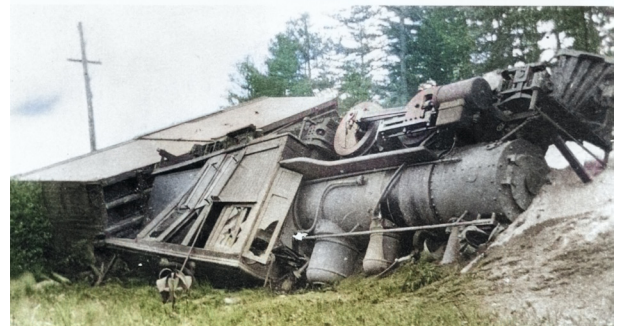
Unseasonable hot weather in mid-May of 1911 caused a sun kink just south of Perley's Mills depot. Engineer could not stop train in time and it came to rest on its side.
